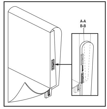
Figure 5. Wing Back Installation
